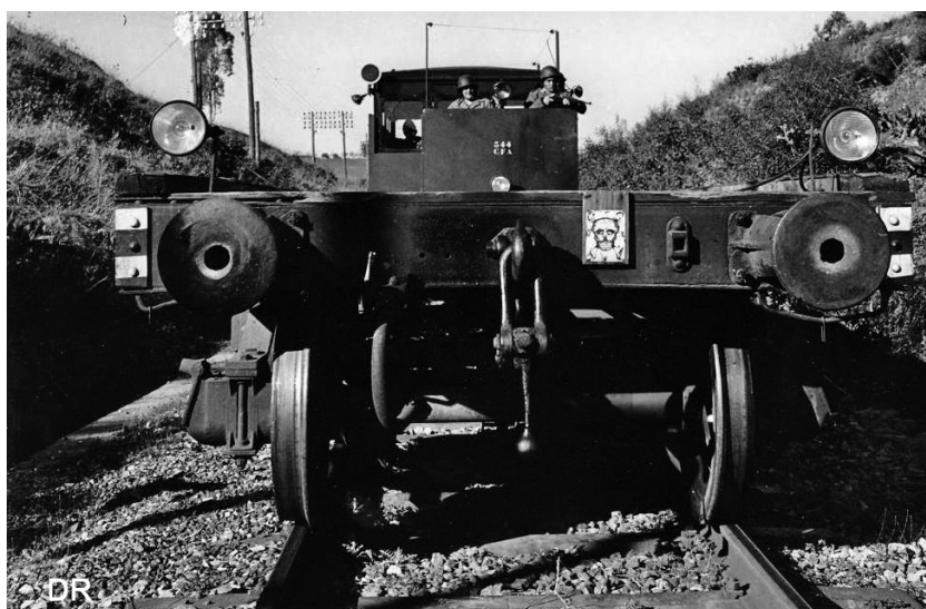
Wagon-plateau anti-mines placé devant la locomotive.
